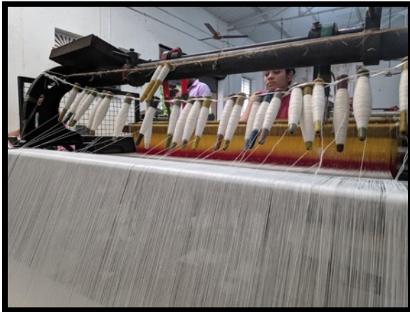
Solar-powered paddle loom, Gondal, Gujarat
